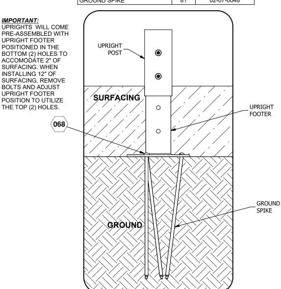
**IMPORTANT:** Never install play equipment over hard, unresilient surfaces such as asphalt, concrete, or compacted earth. It is the owner's responsibility to ensure the "minimum area required" contains an appropriate amount of resilient material to cushion accidental falls.
