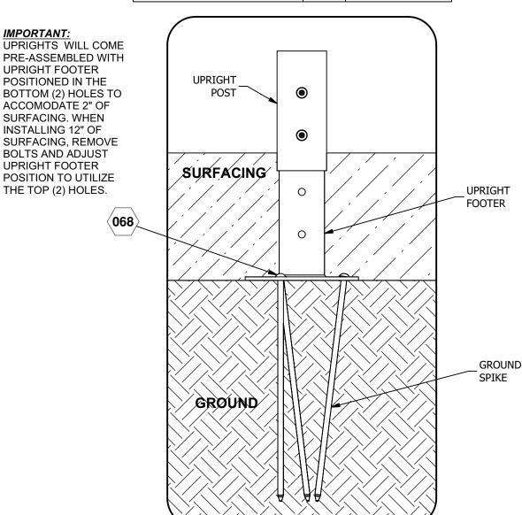
**IMPORTANT:** Never install play equipment over hard, unresilient surfaces such as asphalt, concrete, or compacted earth. It is the owner's responsibility to ensure the "minimum area required" contains an appropriate amount of resilient material to cushion accidental falls.
