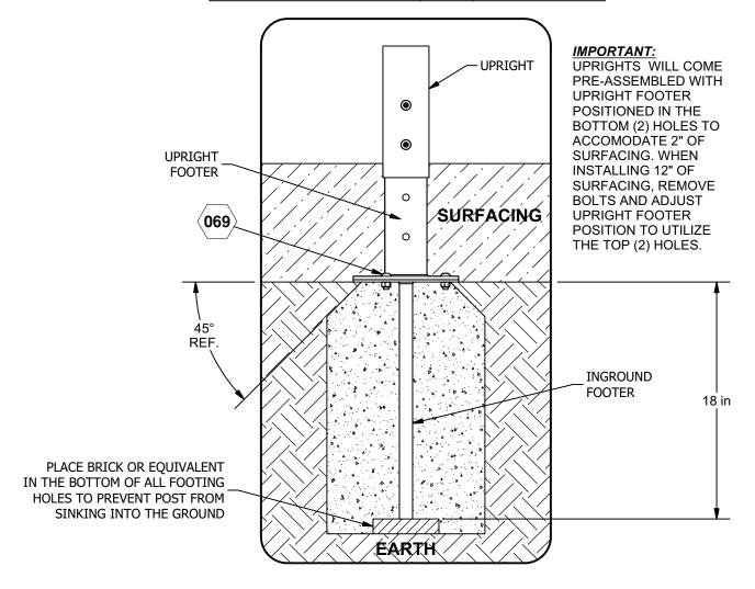
**IMPORTANT:** Never install play equipment over hard, unresilient surfaces such as asphalt, concrete, or compacted earth. It is the owner's responsibility to ensure the "minimum area required" contains an appropriate amount of resilient material to cushion accidental falls.
