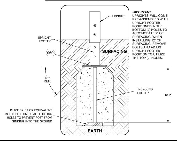
**IMPORTANT:** Never install play equipment over hard, unresilient surfaces such as asphalt, concrete, or compacted earth. It is the owner's responsibility to ensure the "minimum area required" contains an appropriate amount of resilient material to cushion accidental falls.
