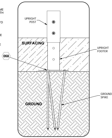
**IMPORTANT:** Never install play equipment over hard, unresilient surfaces such as asphalt, concrete, or compacted earth. It is the owner's responsibility to ensure the "minimum area required" contains an appropriate amount of resilient material to cushion accidental falls.
