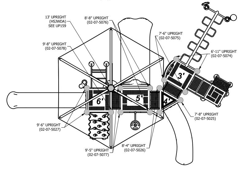
**IMPORTANT:** Fabric Shade UP159 must be installed **In Ground Only.**
