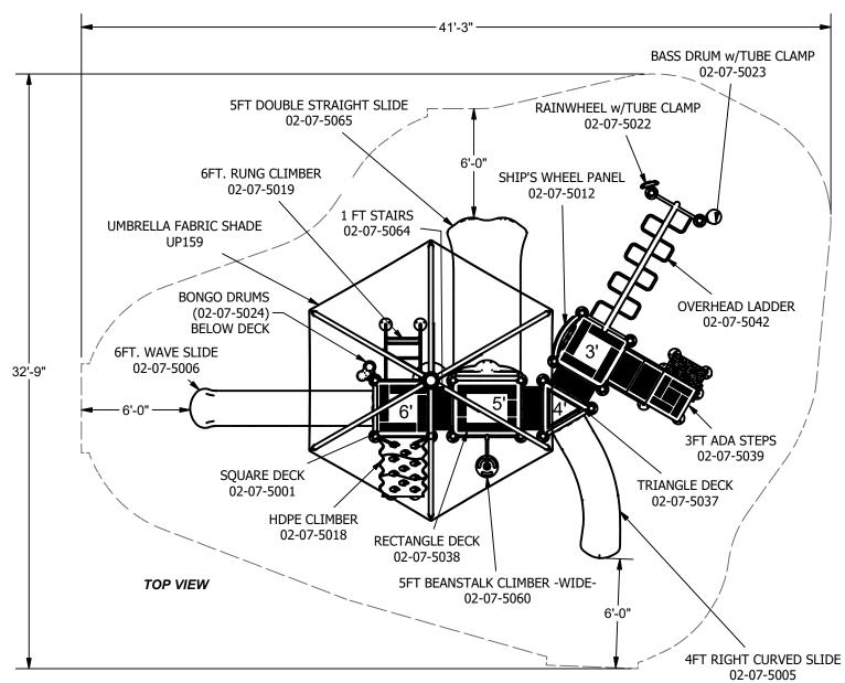
**IMPORTANT:** Fabric Shade UP159 must be installed **In Ground Only.**
