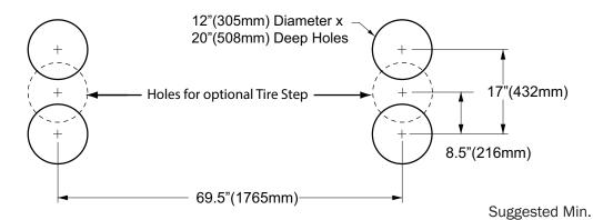
**Concrete Required:** Approx. .2 Cubic Yards (.15 Cubic Meters) Concrete Required (with optional Tire Step): Approx. .3 Cubic Yards (.25 Cubic Meters)
