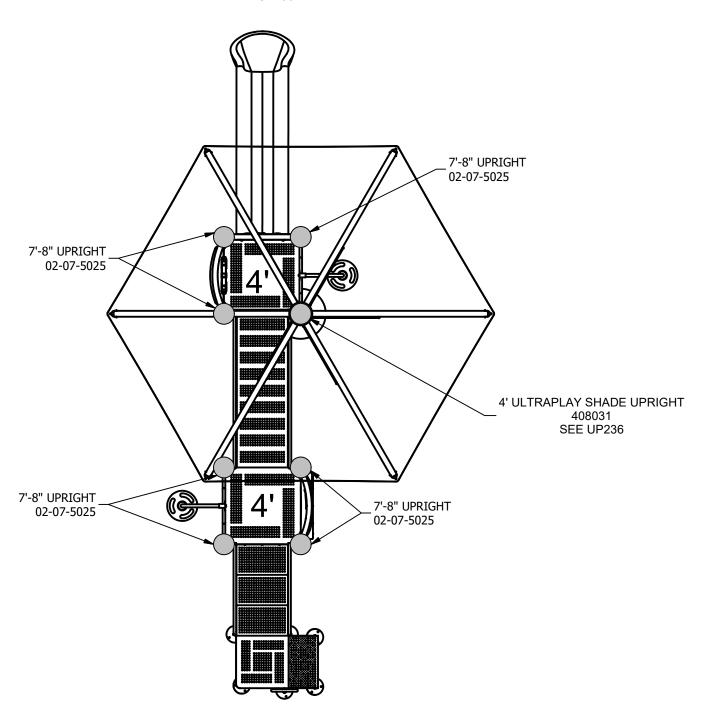
IMPORTANT: Fabric Shade UP236 must be installed In Ground Only.
