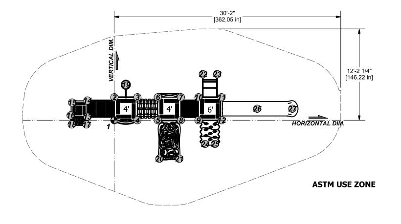
IMPORTANT: Never install play equipment over hard, unresilient surfaces such as asphalt, concrete,or compacted earth. It is the owner's responsibility to ensure the "minimum area required" contains an appropriate amount of resilient material to cushion accidental falls.
