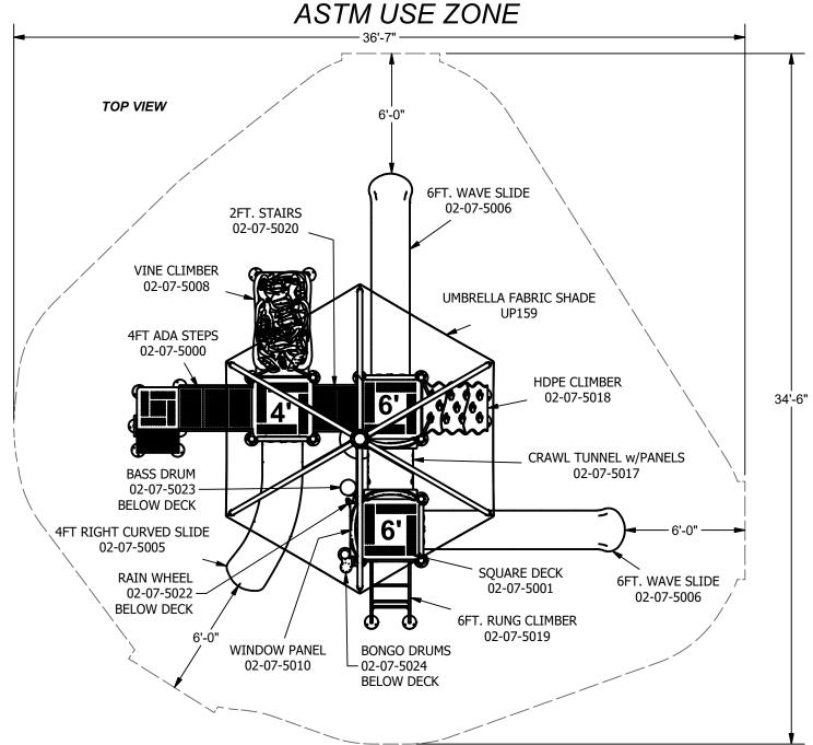
**IMPORTANT:** Fabric Shade UP159 must be installed **In Ground Only.**
