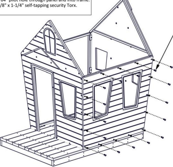
Drill 21/64" Pilot Hole Secure with 3/8" x 1-1/4" Self-Tapping Security Torx Typ. 16
